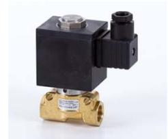
The power consumption of this valve is 16W/20VA, which is relatively high. The heat emission will be significant so the coil needs to be large.
