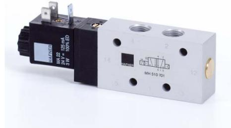
Spool valves can combine a high flow (large orifice size) at a significant maximum pressure (the standard is around 10 bar, can be larger on request) with a low power consumption. In order to function correctly, the valves require **a minimum pressure**. If there is less pressure applied to the valve, the spool might not move. In this case the friction is too high.
